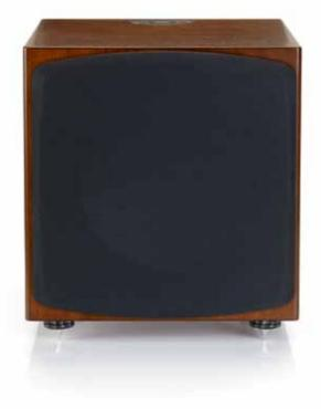
Using the latest switch mode power conversion techniques, the RXW-12's 500 watt Class D amplifier provides enough power to control with brutal efficiency a newly designed 12" C-CAM driver, equipped with a double stack (two magnet) motor system and a massive 3" voice coil.
